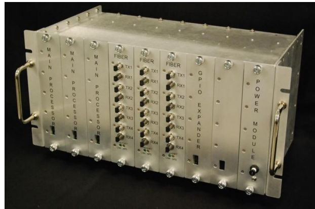
Chassis with Modules Installed – RG Configuration
